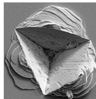
*Nano-impact of a layered  $Cr_2AlC$  MAX-phase coating.*
