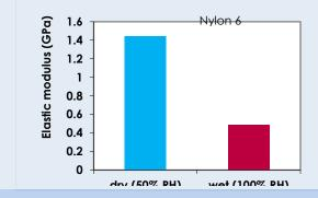
Figure 4 shows that when hydrolytic attack and plasticization occurs, polymer stiffness decreases significantly [...see also G.A Bell, DM Bielinski and BD Beake, J ApplPolymSci 107(2008) 577].
