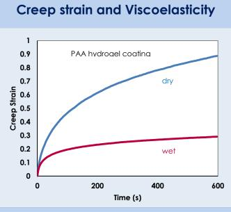
Figure 7 shows that in liquid there is an increase in indentation creep over 600 s. With the high level of stability of The NanoTest Vantage it is possible to look at time dependent properties over long contact times without loss of accuracy from thermal drift.
