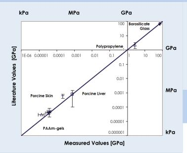
Figure 3 shows the measured Elastic modulii of various specimens (Borosilicate glass, Polypropylene, Porcine liver, Porcine skin, PAAmgels in various mol concentrations) are in very good agreement with literature values. Data ranges over eight orders of magnitude.
