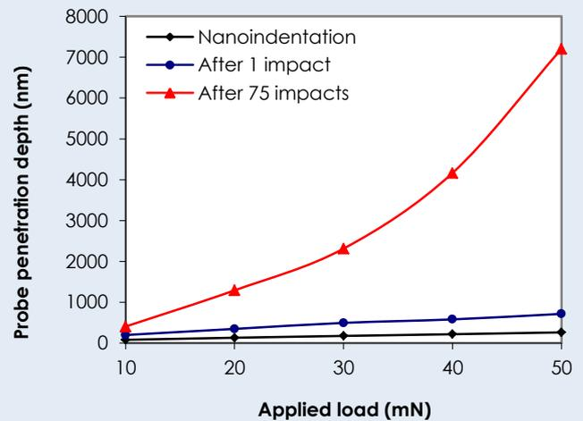
Figure 5 shows a comparison of maximum probe depth after nanoindentation and single and multiple impacts with a 5 μm spherical indenter on thin amorphous hard carbon film on Si shows the penetration depth is much greater in Nano-Impact.
