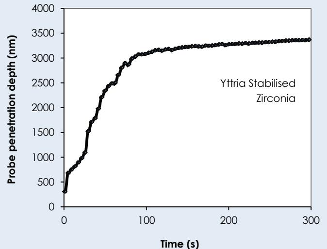
Figure 3 shows repetitive nano-impact tests on a 7-8% Yttria Stabilised Zirconia (thermal barrier coating) that was previously aged for 24 hr at 1500 °C. The rapid nano-impact test shows the decreased resistance to multiple impacts after thermal ageing of the TBC consistent with results from erosion tests.
