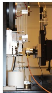
Figure 2 Implementation of AE monitoring in the NanoTest and schematic of AE waveform
