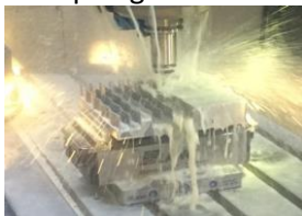
Fig. 1. Trochoidal rough milling of undulated grooves in Inconel 718.
