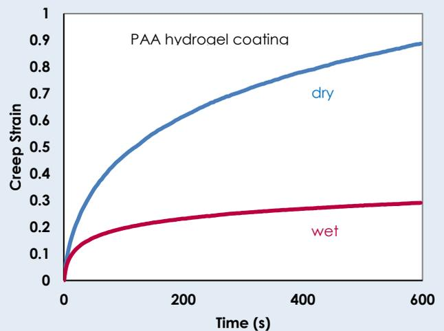
Figure 7 shows that in liquid there is an increase in indentation creep over 600 s. With the high level of stability of The NanoTest Vantage it is possible to look at time dependent properties over long contact times without loss of accuracy from thermal drift.
