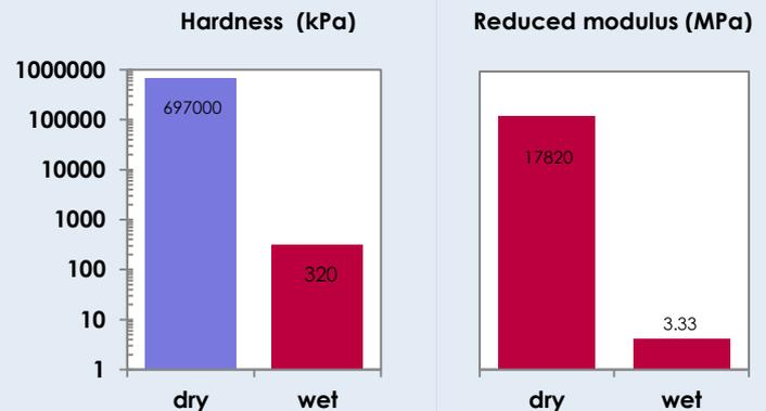
Figure 5 shows that with nanoindentation of a PAA hydrogel in water, the hardness value dropped to the kPa level within minutes of submersion. Similarly the modulus values of the hydrogel are 5300 times lower in water.
