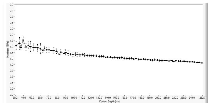
Depth dependence of hardness for Cu(100) single crystal from DMCT – note the absence of any anomalous results or data variability at low depths. The data show mean values from 3 repeat tests.
