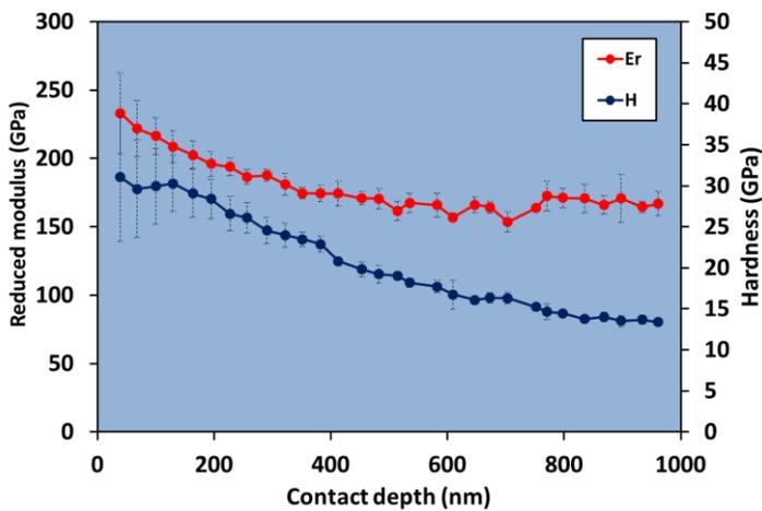
Variation in hardness and reduced modulus with contact depth from continuous stiffness measurements to 300 mN on a 750 nm thick DLC coating on a silicon wafer. The mean values were from 10 experiments.
