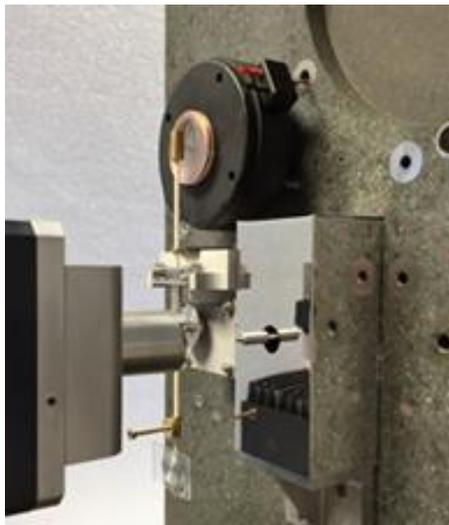
A NanoTest Vantage system showing permanently mounted standard (left) and DMCT (right) 500 mN load heads
