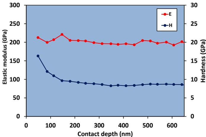
*Hardness and elastic modulus vs. depth at 200 °C in a high carbon martensitic steel from a DMCT experiment to 100 mN with a cBN Berkovich indenter*
