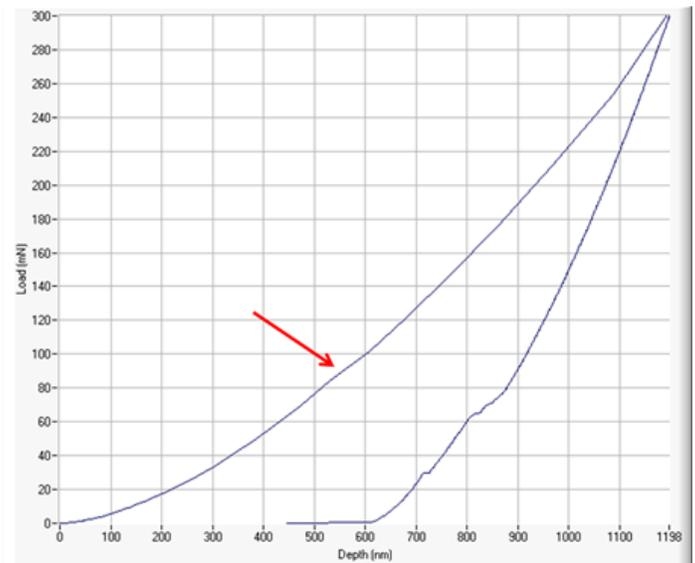
A typical indentation curve showing inflexion during loading (marked with red arrow) and phase transformation during unloading.
