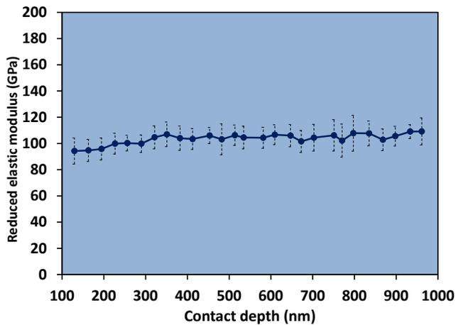
Depth dependence of elastic modulus for a copper sample. The mean values from 10 measurements are shown.
