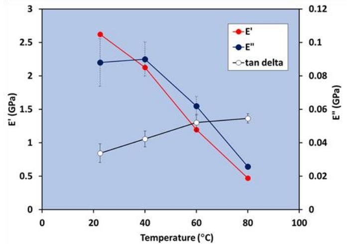
Variation in loss modulus, storage modulus and tan delta with temperature over 22-80 °C
