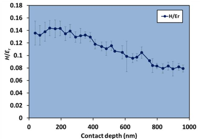
Variation in (hardness/reduced modulus) with increasing contact depth from continuous stiffness measurement.
